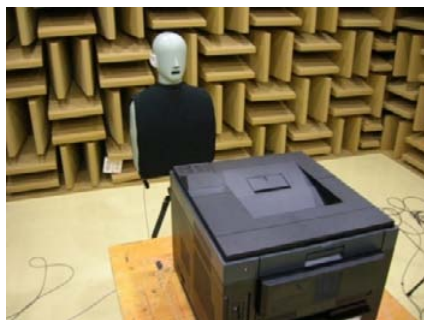
Fig. 16. Measurement of sound quality level of a laser beam printer in a semi-anechoic chamber.
