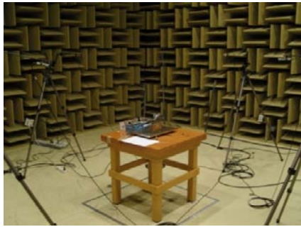
Fig. 14. Measurement of SPL of the experimental gear jig in a semi-anechoic chamber.
